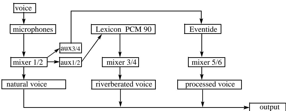
The console must have at least 6 balanced input channels (2 with phantom +48V), one stereo output and 4 stereo auxiliary outputs, two of them with pre-fade option.
